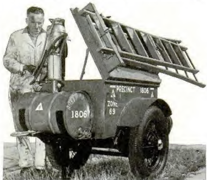
This fire fighting trailer carries along its own water supply
